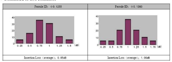
• Connected to bare fiber adapter
